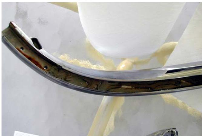
When cleaning the upper and lower frame assemblies, pay attention to the floating anchor plates found at each end of the frame assemblies. These pieces have threaded holes where the screws removed from the side post assemblies attach. In both cases (upper and lower), these pieces will be immersed in the putty and won’t be immediately noticeable.
