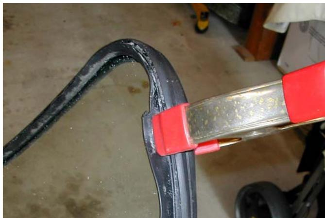
As I mentioned I've had this rubber channel for a number of years and new ones may fit differently. However, in this case I found that I had to stretch the rubber substantially to get it to fit. **Remember Rule 1.** So, I carefully stretched the rubber as I installed it so that the bottom centers remained in agreement and the rubber encircled the window.
