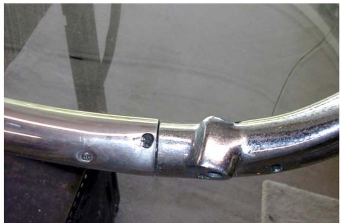
Once the four screws are out, grasp the top of the side post assembly and try to pull it apart from the top frame assembly. If it moves, just pull it out ¼” or so. Then grasp the bottom of the side post assembly and try to pull it out of the bottom frame assembly. As above, if it
