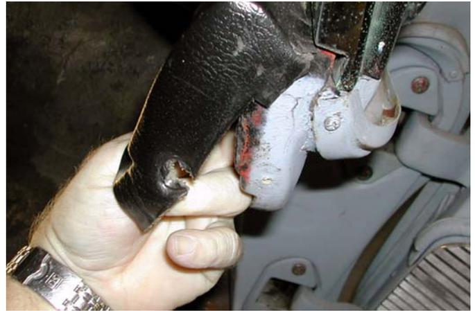
Somewhere in a previous life, someone had the windshield off this car because they had enlarged the access hole so that it is easier to get to the nuts. You can see where the hole was cut with – probably, a key hole saw. Not very professional, but access to the nuts must really be difficult without that hole being enlarged. Once the four 1/2" nuts are removed from the side frame assemblies, the hard part starts.
