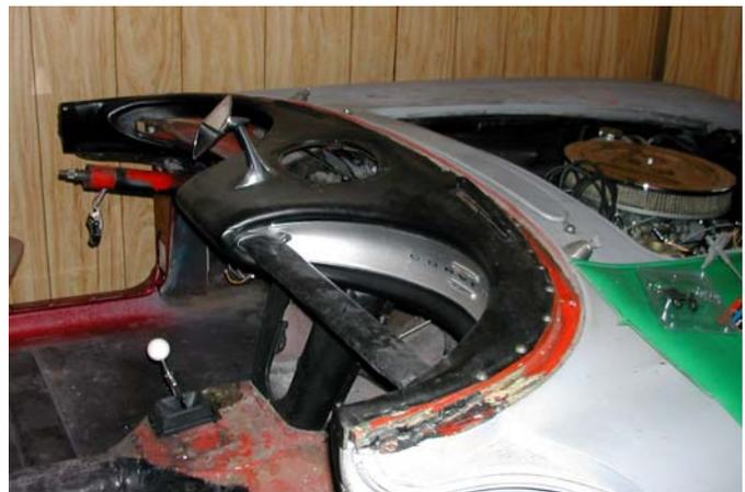
Once the frame is loose from the body, lay it face down on a padded saw horse or suitable work bench. Handle this thing carefully, the frame provides only moderate support to the
