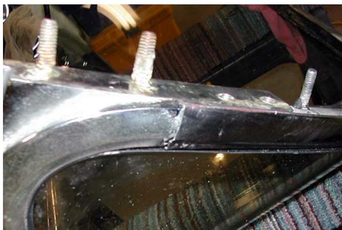
Be very careful, while there is a rubber channel gasket between the floating anchor and the glass of the window it is possible to get heavy handed and push a sharp scribe through the rubber and scratch the edge of the glass – if this happens – most certainly the glass will crack! (Been there, done that!!!)
