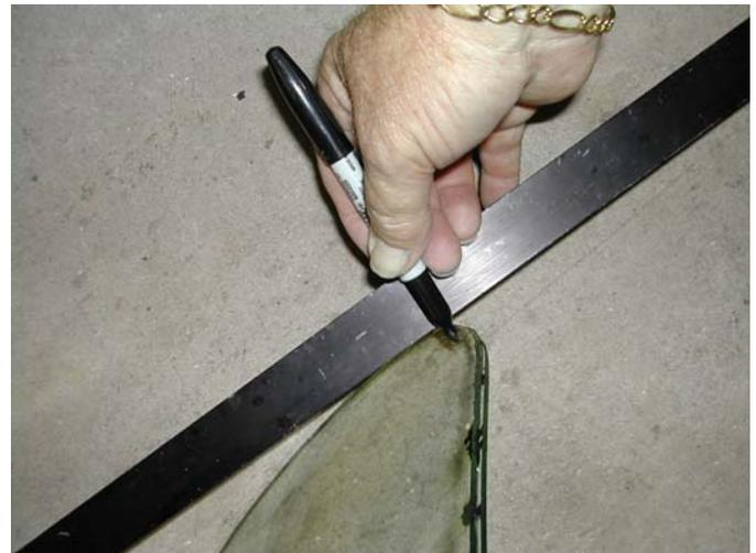
After that it was merely a matter of measuring from the marked spots to the center of the bottom of the windshield. For installation of the rubber channel I don't believe it is necessary to mark the center of the top of the windshield. However, a top center mark will be helpful when remounting the upper frame assembly.
