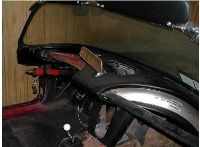
The windshield frame is held to the car body with a total of 12 bolts – two bolts at each end are actually studs (5/16X18) in the side frame assembly. The picture at the right shows those studs – obviously, in this picture the frame is already off the car – it makes it easier to see how the bolts are set up.
