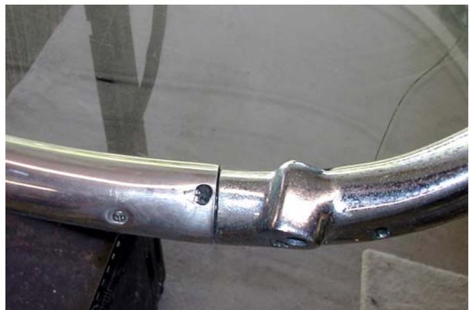
Once the four screws are out, grasp the top of the side post assembly and try to pull it apart from the top frame assembly. If it moves, just pull it out ¼” or so. Then grasp the bottom of the side post assembly and try to pull it out of the bottom frame assembly. As above, if it
